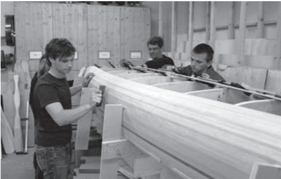
Carpentry workshop at the VHS Cham: building a canoe
